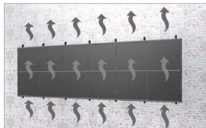
Very good rear ventilation of the modules
